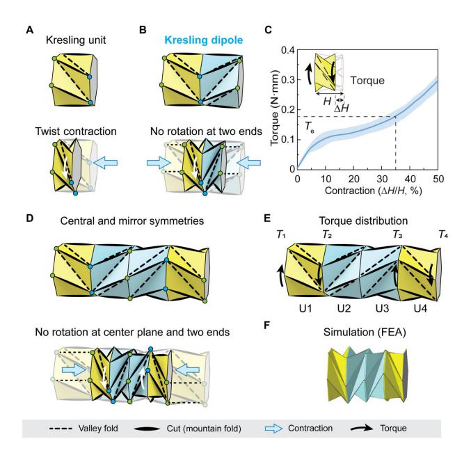
Mechanism of the four-unit Kresling crawler based on the Kresling dipole. (A) Schematic of a Kresling unit, showing contraction coupled with a twist
