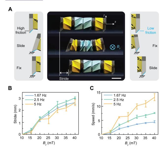
Crawling mechanism of the Kresling robot. (A) Single stride of the Kresling crawler under a magnetic field of 40 mT. Scale bar, 5 mm. (B) Stride and (C) speed characterization of crawling motion at various magnetic field magnitudes and frequencies. Credit: *Science Advances* (2022). DOI: 10.1126/sciadv.abm7834
