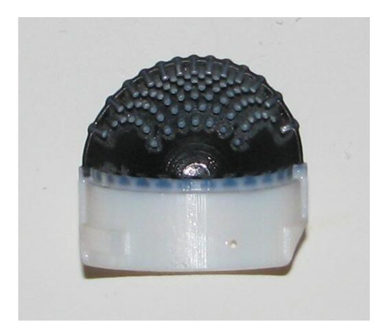
Cut-through section on the 3D-printed tactile skin. The white plastic is a rigid mount for the flexible black rubber skin. Both parts are made together on an advanced 3D-printer. The 'pins' on the inside of the skin replicate dermal papillae that are formed inside human skin. Credit: Prof. Nathan Lepora
