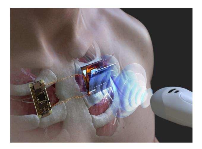
Schematic illustration of wirelessly charging a body-implanted electronic device using an ultrasonic probe. Credit: Korea Institute of Science and Technology (KIST)
