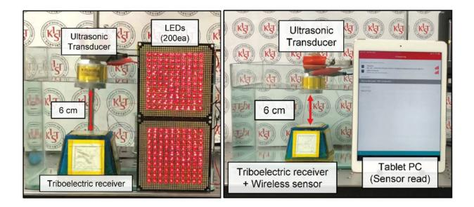
Underwater wireless acoustic energy transfer system that can simultaneously operate 200 LEDs and a wireless sensor in real time. Credit: Korea Institute of Science and Technology (KIST)
