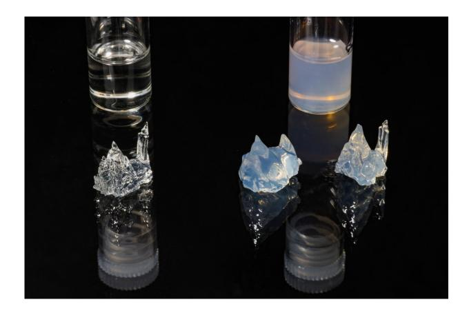
Three 3D-printed objects: one made from transparent resin (left); one from opaque resin, without correction (middle); and one from opaque resin, with correction (right). Credit: © Alain Herzog 2022 EPFL
