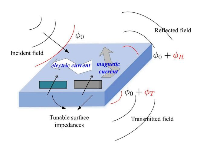
Schematic illustration of the simultaneously transmitting and reflecting RIS element. Credit: Intelligent and Converged Networks
