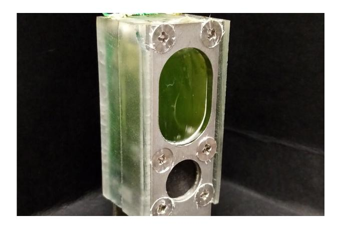
This system, containing blue-green algae, powered a microprocessor continuously for a year using nothing but ambient light and water. Credit: Paolo Bombelli
