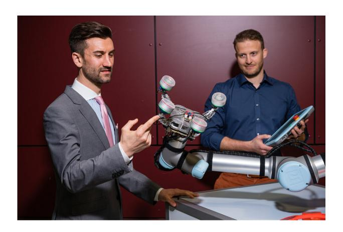
The robot gripper designed by Stefan Seelecke and his team can grip objects with complex geometries and can adapt to changes in form, switching seamlessly between differently shaped parts. Paul Motzki (l.) and Lukas Zimmer (r.) helped develop the system. Credit: Oliver Dietze
