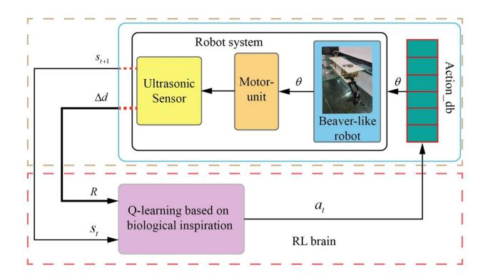
Training controller structure of the robot. Credit: *Robotics and Autonomous Systems* (2022). DOI: 10.1016/j.robot.2022.104116
