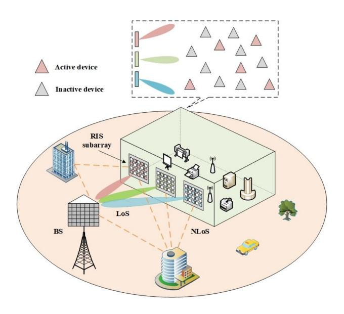
Illustration of an RIS-assisted grant-free massive access in a smart factory, where a cluster of RIS subarraysworking in the refraction mode are deployed on the
