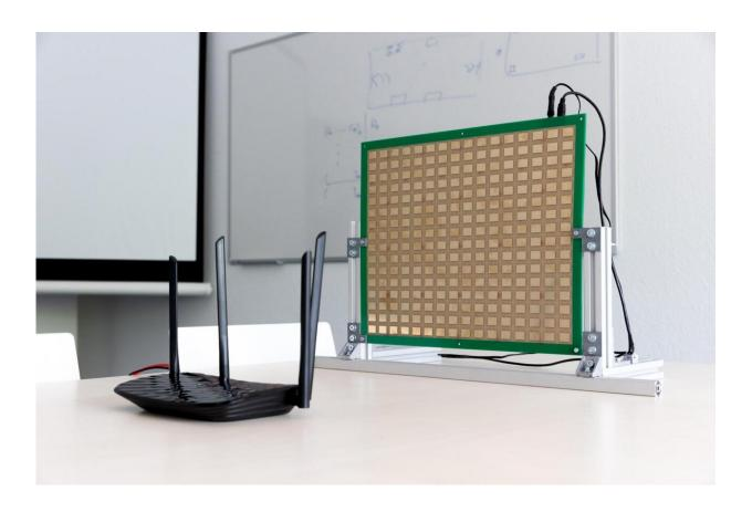
The intelligent reflecting surface IRShield is positioned next to a Wi-Fi router for obfuscation of the environment-dependent wireless channel. Credit: CASA, Michael Schwettmann
