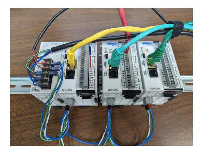
SwRI used programmable logic controllers (PLCs) connected to input/output (I/O) modules to a test network. Algorithms scanned the network for cyberattacks through data packets transferred over the Modbus/TCP protocol. Credit: Southwest Research Institute
