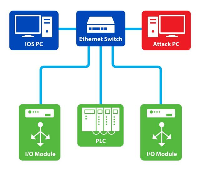
SwRI designed an industrial network to detect cyberattacks from a malicious computer. The network utilized the Modbus/TCP protocol to transfer data packets between input/output (I/O) devices and programmable logic controllers (PLCs) connected via an Ethernet switch. Credit: Southwest Research Institute
