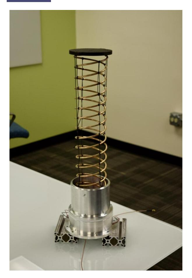
The helical antenna in its fully deployed state. Credit: University of Colorado at Boulder
