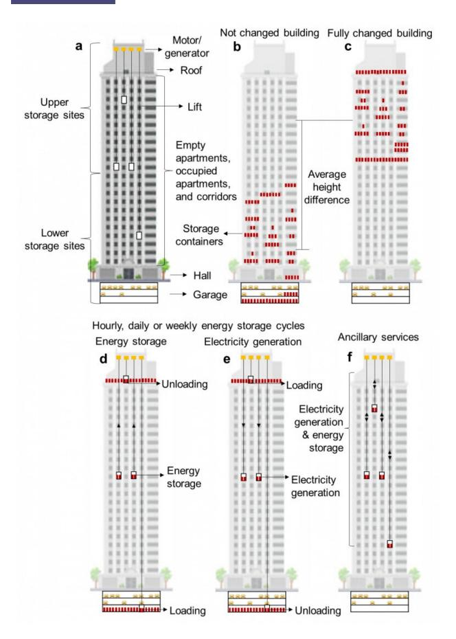
Lift Energy Storage Technology (LEST) (a) system components, (b) not changed and (c) fully charged building, (d) operating on energy storage, (e) electricity generation, or (f) ancillary services mode. Credit: *Energy* (2022). DOI: 10.1016/j.energy.2022.124102
