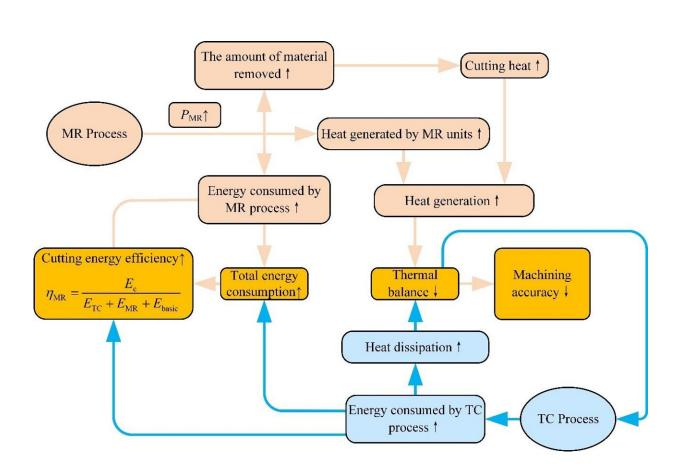
Coupling relationship between the MR process and TC process of machine tools. Credit: Kexu Lai , Huajun Cao , Hongcheng Li , Benjie Li , Disheng Huang
