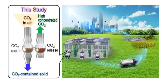
Atmospheric air with low concentrations of carbon dioxide is passed through an aqueous solution of IPDA, where the carbon dioxide rapidly reacts to create a solid product. Carbon dioxide is subsequently re-released with mild heating of the product in suspension, for storage or new applications. Credit: Tokyo Metropolitan University
