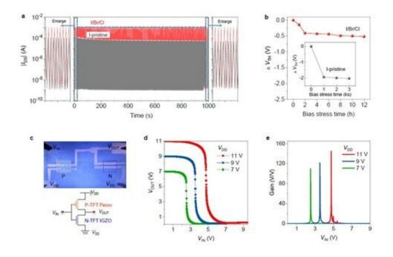
Operating stability of perovskite TFTs and performance of the integrated inverters.(a) Consecutive on/off switching test of iodine-based and iodine/bromine/chlorine-based TFTs (b) Threshold voltage change with respect to bias VGS = VDS = -12 V (c) Perovskite/IGZO inverter (d) Voltage transfer (e) Gain. Credit: POSTECH
