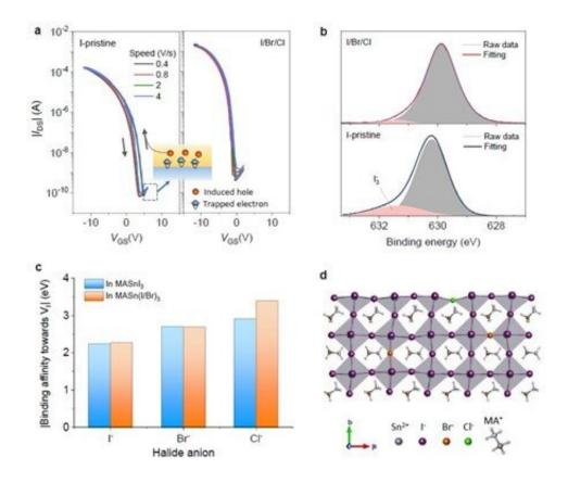
Analysis of hysteresis and iodine attack point of  $MASnI_3$  perovskite TFTs(a) Iodine-based, iodine/bromine/chlorine-based thin film transistor performance as a function of scan rate (b) I 3d3/2 X-ray optical spectrum (c) Halide anion and iodine according to  $MASnI_3$  and  $MASn(I/Br)_3$  interaction strength between defects (d) Passivation effect of iodine defect by a chlorine anion. Credit: POSTECH
