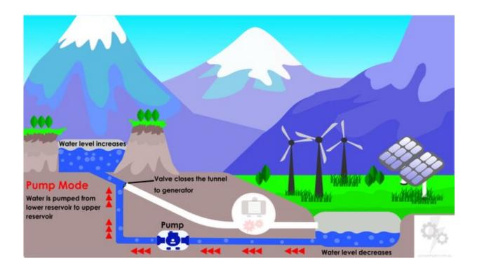
Pumped hydro energy storage in pumping mode. Credit: pumpedhydro.com.au
