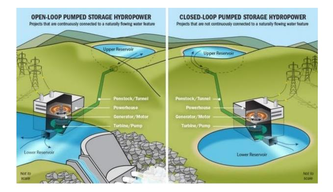
Two types of pumped-storage hydropower: river-based (left) and off-river (right). Credit: NREL
