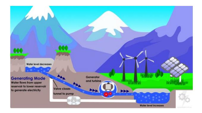
Pumped hydro energy storage in generating mode. Credit: pumpedhydro.com.au
