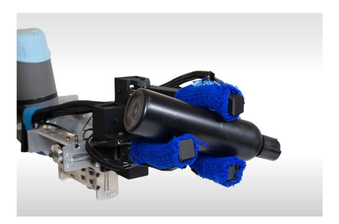
MIT researchers have created an integrated design pipeline that enables a user with no specialized knowledge to quickly craft a customized 3D-printable robotic hand. Credit: Lara Zlokapa
