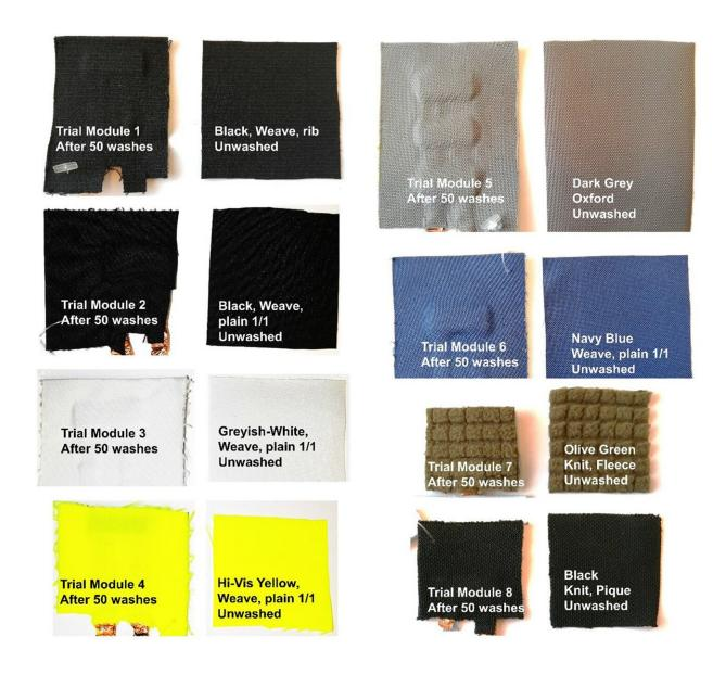
Textile solar modules before (right) and after 50 cycles of washing (left). Credit: *Research Journal of Textile and Apparel* (2022). DOI: 10.1108/RJTA-01-2022-0004
