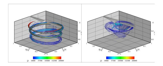
Wake structures produced by rotary wings: left, helical shape imposed by strong tip vortices of traditional rotor; right, conical shape by weak vortex strength of quiet rotor. Credit: University of Illinois Dept. of Aerospace Engineering
