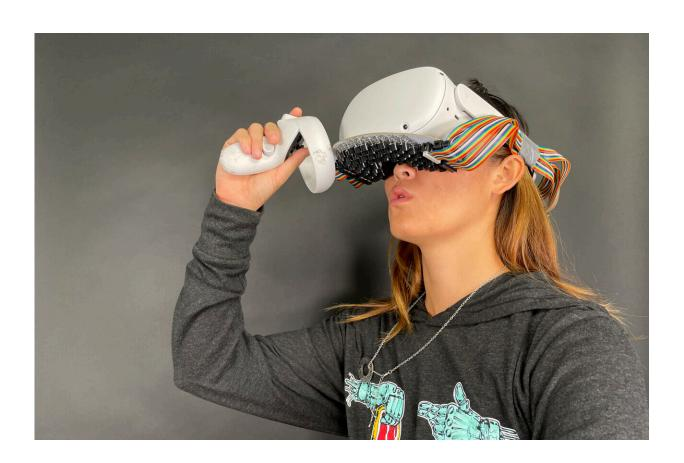
Vivian Shen, a Ph.D. student in Carnegie Mellon University's Robotics Institute, uses a virtual reality headset equipped with a phased array of ultrasound transducers to simulate the feeling of drinking on her lips. Credit: Carnegie Mellon University
