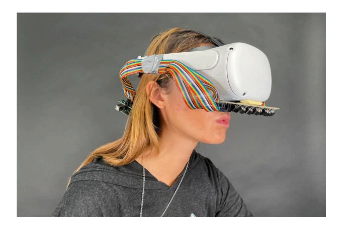
Vivian Shen, a Ph.D. student in Carnegie Mellon University's Robotics Institute, uses a virtual reality headset equipped with a phased array of ultrasound transducers that provide haptic feedback on the mouth. Credit: Carnegie Mellon University
