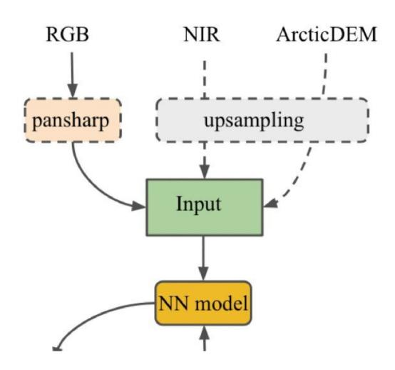
Experiment workflow for canopy height estimation by utilization of deep neural networks, different configurations of input data, various spectral compound, spatial resolution and topography features. The dotted lines show optional steps for input tensor creation. Credit: *IEEE Access* (2022). DOI:
