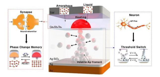
Neuromorphic memory device consisting of bottom volatile and top nonvolatile memory layers emulating neuronal and synaptic properties, respectively. Credit: The Korea Advanced Institute of Science and Technology (KAIST)
