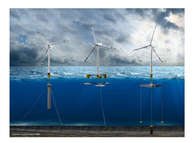
Floating offshore wind turbines require unique mooring systems to hold them in place, which can increase the space needed for wind power plant development. Classic floating platform concepts can include spar (left), semisubmersible (center), and tension leg platforms (right). Credit: Joshua Bauer, NREL
