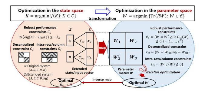
The schematic illustration of the proposed structured optimal control method. Credit: NIMTE
