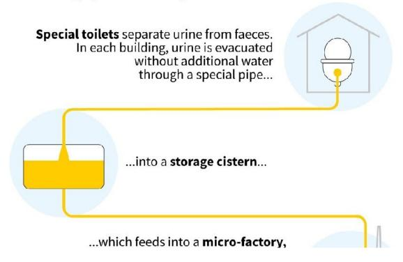
Graphic showing a process transforming urine into fertiliser.
