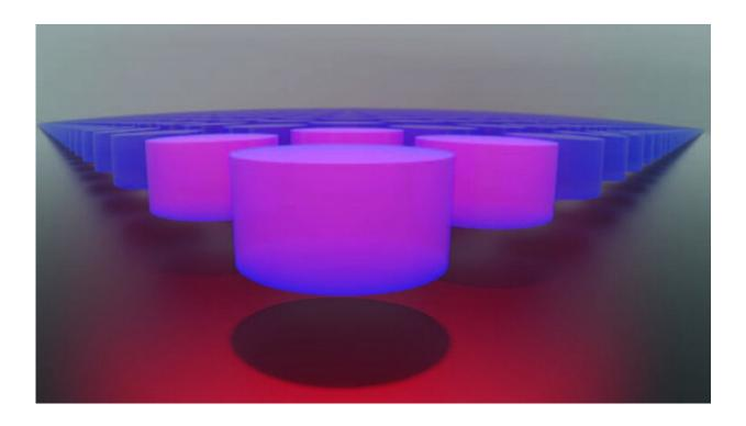
Silicon metamaterials such as this, featuring rows of cylinders extending into the distance, can manipulate light depending on the features of the cylinders. Research has now shown that incorporating known physics into a machine learning algorithm can reveal new insights into how to design them. Credit: Duke University
