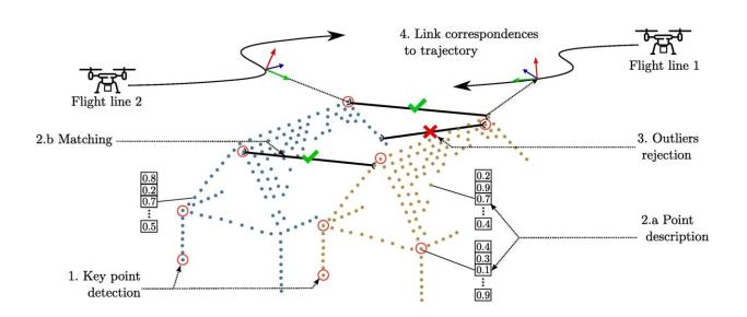
Overview of steps to connect trajectories via lidar pulse observations through the key point-to-point detection and matching principle. Two overlapping and misaligned lidar point clouds in blue and orange are related to a portion of two overlapping flight lines 1 and 2. Credit: *ISPRS Journal of Photogrammetry and Remote Sensing* (2022). DOI: 10.1016/j.isprsjprs.2022.04.027
