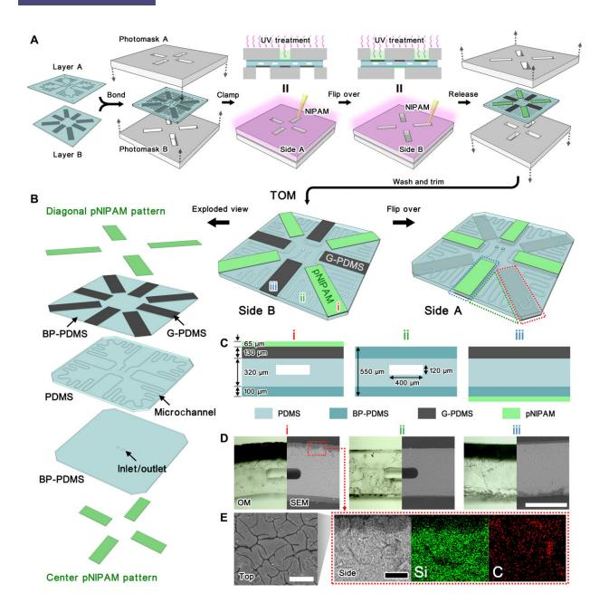
Fabrication and characterizations of TOM. (A) Fabrication of TOM. (B) Schematics show both sides of the final device and the exploded view of TOM. (C) Schematic cross sections of three regions on TOM. (D) OM and SEM of three regions. Scale bar, 500  $\mu$ m. (E) SEM imaging on pNIPAM top surface and the interface between pNIPAM and G-PDMS coupled with EDX mapping. Scale bars, 100  $\mu$ m. Credit: *Science Advances* (2022). DOI: 10.1126/sciadv.abo1719
