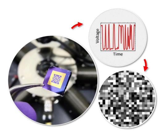
The image of the fabricated electronic chip that generates the random number. The chip is loaded into the measurement setup, where the randomness of the electron trapping/de-trapping is converted into binary outputs. Credit: Nithin Abraham
