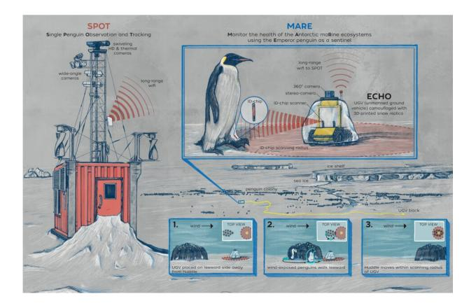
An illustration of the remote-controlled ground robot, ECHO. Credit: Woods Hole Oceanographic Institution
