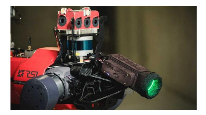
The GLIMPSE robot has instruments for petrographic and chemical rock analysis, including a Raman spectrometer, a microscope and a camera with zoom lens for overview and close-up images. Credit: Team Glimpse
