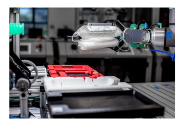
The Swinburne team has designed a robot arm to automate the blood donation pack folding process. The arm holds the folded blood pack, which is filled with water, to demonstrate that this process can be automated.
