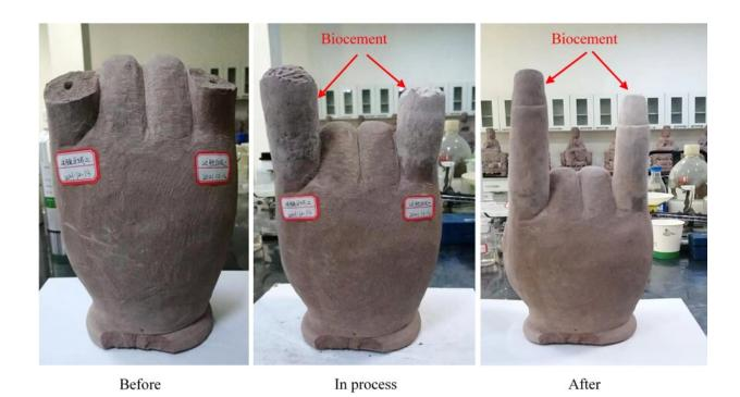
The test specimen of a Buddha hand was provided by Dazu Rock Carvings, a UNESCO World Heritage Site in China. Repair work using biocement was done at Chongqing University, China, by Dr Yang Yang. The biocement solution is colourless, allowing restoration works to maintain the carving's original colour. Credit: Nanyang Technological University
