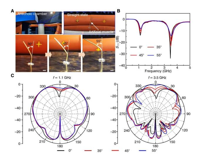
Application of the multifunctional artificial muscle as a reconfigurable antenna: (A) Different bending angles of the multifunctional artificial muscle after first,
