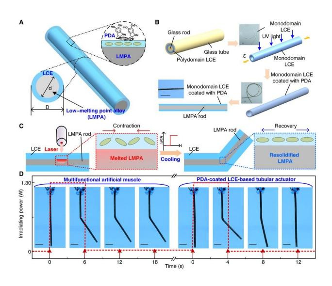
Multifunctional artificial muscle composed of PDA-coated tubular LCE and LMPA rod. (A) Multifunctional artificial muscle consisted of tubular LCE
