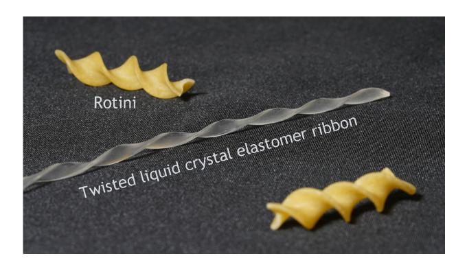
Researchers have developed soft robots that are capable of navigating complex environments, such as mazes, without input from humans or computer software. The soft robots are made of liquid crystal elastomers in the shape of a twisted ribbon, resembling translucent rotini. Credit: Yao Zhao, NC State University
