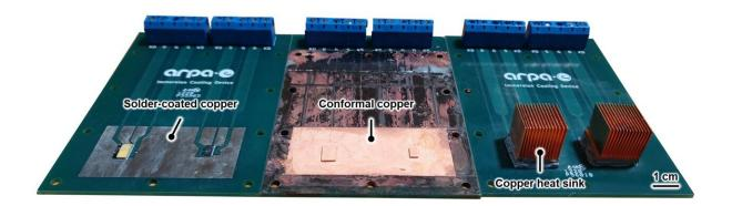
The copper coating heat spreader developed in this study (center) compared to two standard thermal management methods: a printed circuit board (PCB) solder-coated copper plane (left), and a copper heat sink (right). Credit: Gebrael et al.
