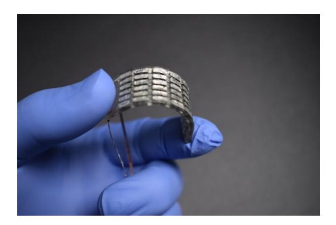
A transducer combining liquid crystal elastomers with a thermoelectrical device provides advantages like active cooling and regenerative energy harvesting for soft robotics. Credit: Soft Machines Lab, Carnegie Mellon University
