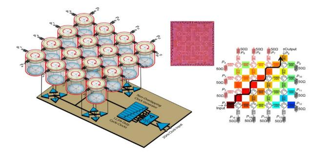
First Floquet topological insulator on an integrated circuit. Arrows shows how transistors are used to achieve non-reciprocity. Credit: Aravind Nagulu
