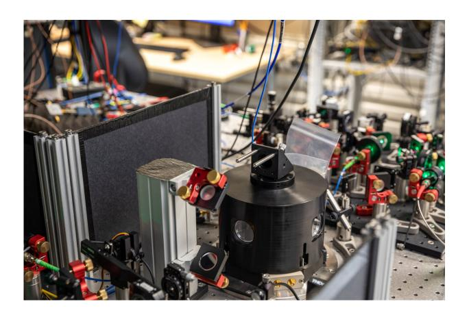
Alice, the receiver of the teleported quantum information. Inside the black aluminium cylinder, the diamond sample is cooled to -270°C, to reduce the noise from the environment and enable the quantum control. Credit: Marieke de Lorijn for QuTech
