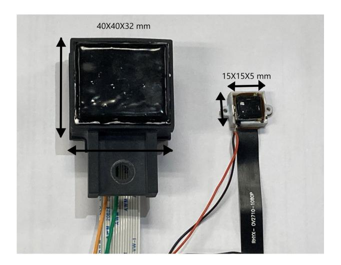
The team's minimized tactile sensor and a normal-sized vision-based tactile sensor. Credit: Chen et al.
