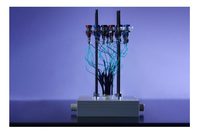
Custom experimental setup used to characterize 30 glucose fuel cells in rapid sequence. Credit: Kent Dayton
