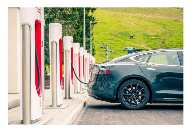
A Tesla EV can travel up to 200 miles (322 km) with 15 minutes of charging at a Tesla Supercharger. Destination chargers are slower to charge - 44 miles (71 km) per hour of charging. Hotels more commonly host Destination charging stations than Superchargers. Credit: Jakob Härter
