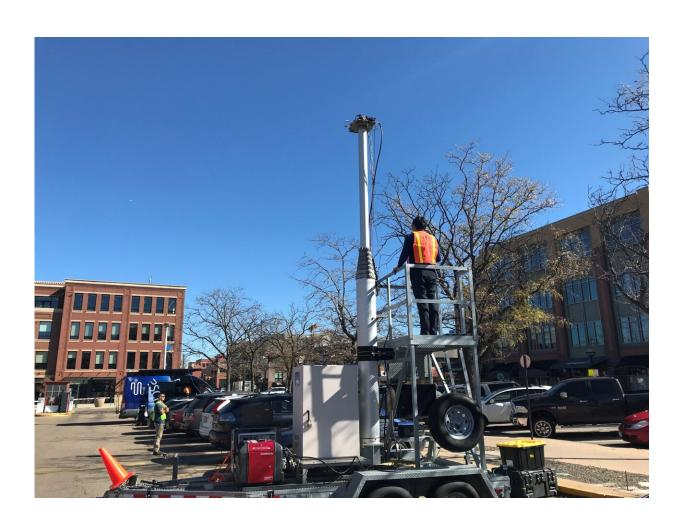
NIST communications researchers traveled to downtown Boulder, Colorado, to verify their channel model for evaluating high-frequency wireless network designs. Sung Yun Jun is checking the alignment of the transmitter, mounted 6 meters high on a mast, with the receiver antenna array on the roof of the blue van. Derek Caudill, barely visible inside the van, is preparing software programs to collect measurement data. Justin Sadinski, in a yellow vest, is checking
