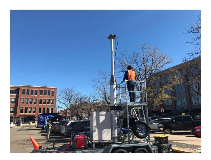
NIST communications researchers traveled to downtown Boulder, Colorado, to verify their channel model for evaluating high-frequency wireless network designs. Sung Yun Jun is checking the alignment of the transmitter, mounted 6 meters high on a mast, with the receiver antenna array on the roof of the blue van. Derek Caudill, barely visible inside the van, is preparing software programs to collect measurement data. Justin Sadinski, in a yellow vest, is checking
