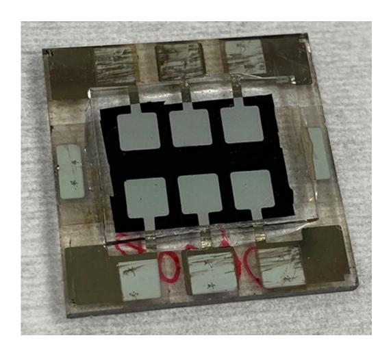
Researchers were able to fabricate this perovskite solar cell that overcomes problems with stability. Credit: National Renewable Energy Laboratory
