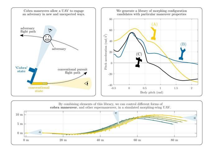
Supermanuevers, such as the cobra maneuver, can be of significant use in air-toair combat. Using a library of wing morphing states, a biomimetic morphingwing aircraft can carry out these supermaneuvers. Credit: Pons & Cirak.
