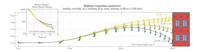
Other supermaneuvers are also available. Illustrated is an example of a ballistic transition maneuver carried out by a biomimetic aircraft: a rapid deceleration and soft landing maneuver on the vertical surface of a building. Credit: Pons & Cirak.
