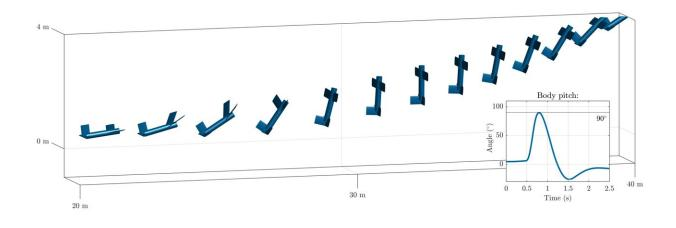
The cobra maneuver is named so because it resembles the rearing of a cobra. Illustrated is a central segment of a simulation of a cobra maneuver carried out by a biomimetic aircraft. Credit: Pons & Cirak.
