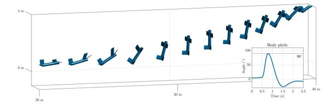
The cobra maneuver is named so because it resembles the rearing of a cobra. Illustrated is a central segment of a simulation of a cobra maneuver carried out by a biomimetic aircraft. Credit: Pons & Cirak.
