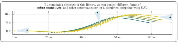
Supermanuevers, such as the cobra maneuver, can be of significant use in air-to-air combat. Using a library of wing morphing states, a biomimetic morphing-wing aircraft can carry out these supermaneuvers. Credit: Pons & Cirak.
