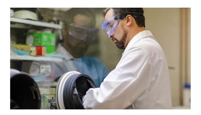
Nuclear engineering doctoral student Sean Martinson works on plutonium solution purification inside a protective glove box in Sunil Chirayath's nuclear forensics laboratory. Credit: Justin Elizalde/Texas A&M Engineering
