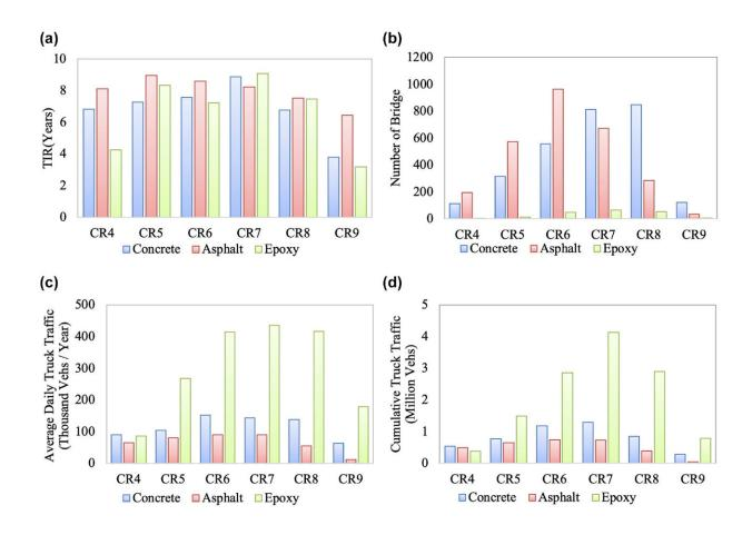
Distribution for surface type by condition rating of: (a) time-in-rating, (b) number of bridges, (c) average daily truck traffic, and (d) cumulative truck traffic. Credit: *Transportation Research Record: Journal of the Transportation Research Board* (2022). DOI: 10.1177/03611981221078281
