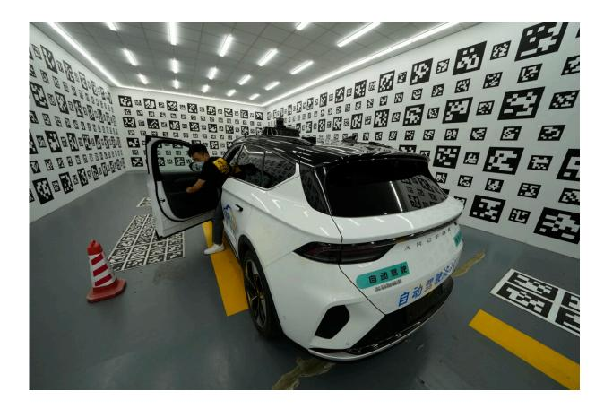
A driver leaves a car after parking it in a chamber used to calibrate the self-driving taxi developed by tech giant Baidu Inc. on June 14, 2022, in Beijing. Baidu Inc. is China's highest-profile competitor in a multibillion-dollar race with Alphabet Inc.'s Waymo and General Motors Co.'s Cruise to create self-driving cars. Credit: AP Photo/Ng Han Guan
