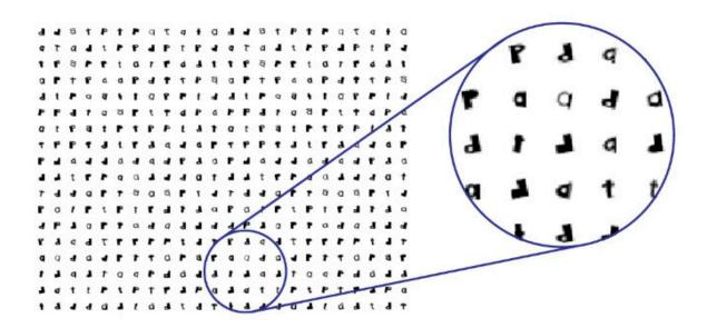
As a proof of concept, the researchers' chip was tested on data sets containing either two or four types of handwritten characters, achieving classification accuracies higher than 93.8% and 89.8%, respectively. Credit: University of Pennsylvania
